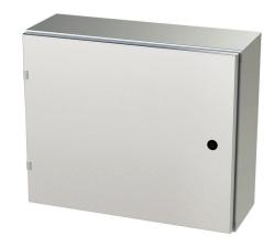
Saginaw Enviroline series enclosure, NEMA 3R/4/4X/12/13,  $20 \times 24 \times 8$  in (HxWxD), wall mount, 304 stainless steel, #4 brush finish, single-door, 1/4-turn semi-flush latch.
