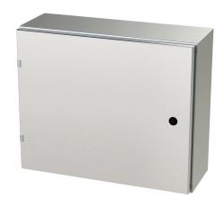
Saginaw Enviroline series enclosure, NEMA 3R/4/4X/12/13, 20 x 24 x 8in (HxWxD), wall mount, 316L stainless steel, #4 brush finish, single-door, 1/4-turn semi-flush latch.
