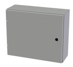
Saginaw Enviroline series enclosure, NEMA 3R/4/12/13,  $20 \times 24 \times 8$  in (HxWxD), wall mount, carbon steel, ANSI 61 gray, powder coat finish, single-door, 1/4-turn semi-flush latch.
