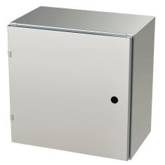
Saginaw Enviroline series enclosure, NEMA 3R/4/4X/12/13, 20 x 20 x 12in (HxWxD), wall mount, 304 stainless steel, #4 brush finish, single-door, 1/4-turn semi-flush latch.
