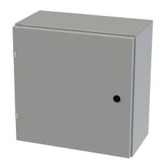
Saginaw Enviroline series enclosure, NEMA 3R/4/12/13, 20 x 20 x 10in (HxWxD), wall mount, carbon steel, ANSI 61 gray, powder coat finish, single-door, 1/4-turn semi-flush latch.
