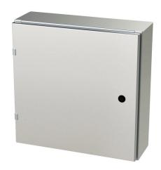
Saginaw Enviroline series enclosure, NEMA 3R/4/4X/12/13,  $20 \times 20 \times 6$  in (HxWxD), wall mount, 304 stainless steel, #4 brush finish, single-door, 1/4-turn semi-flush latch.
