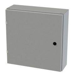
Saginaw Enviroline series enclosure, NEMA 3R/4/12/13,  $20 \times 20 \times 6$  in (HxWxD), wall mount, carbon steel, ANSI 61 gray, powder coat finish, single-door, 1/4-turn semi-flush latch.
