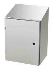
Saginaw Enviroline series enclosure, slope top, NEMA 3R/4/4X/12/13, 20 x 16 x 12in (HxWxD), wall mount, 304 stainless steel, #4 brush finish, single-door, 1/4-turn semi-flush latch.
