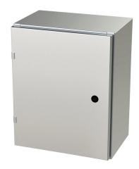
Saginaw Enviroline series enclosure, NEMA 3R/4/4X/12/13,  $20 \times 16 \times 10$  in (HxWxD), wall mount, 316L stainless steel, #4 brush finish, single-door, 1/4-turn semi-flush latch.
