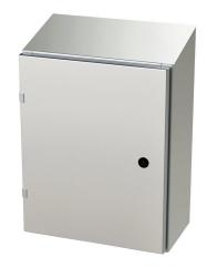
Saginaw Enviroline series enclosure, slope top, NEMA 3R/4/4X/12/13, 20 x 16 x 8in (HxWxD), wall mount, 304 stainless steel, #4 brush finish, single-door, 1/4-turn semi-flush latch.
