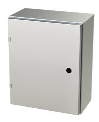
Saginaw Enviroline series enclosure, NEMA 3R/4/4X/12/13,  $20 \times 16 \times 8$  in (HxWxD), wall mount, 316L stainless steel, #4 brush finish, single-door, 1/4-turn semi-flush latch.
