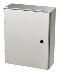
Saginaw Enviroline series enclosure, NEMA 3R/4/4X/12/13, 20 x 16 x 6in (HxWxD), wall mount, 304 stainless steel, #4 brush finish, single-door, 1/4-turn semi-flush latch.
