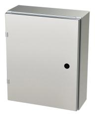
Saginaw Enviroline series enclosure, NEMA 3R/4/4X/12/13, 20 x 16 x 6in (HxWxD), wall mount, 316L stainless steel, #4 brush finish, single-door, 1/4-turn semi-flush latch.
