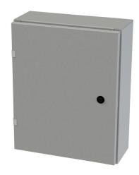
Saginaw Enviroline series enclosure, NEMA 3R/4/12/13,  $20 \times 16 \times 6$  in (HxWxD), wall mount, carbon steel, ANSI 61 gray, powder coat finish, single-door, 1/4-turn semi-flush latch.
