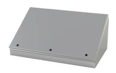
Saginaw operator consolet, NEMA 3R/4/12/13, 20 x 30 x 13in (HxWxD), desktop or pedestal mount, carbon steel, ANSI 61 gray, powder coat finish, single-door, 1/4-turn semi-flush latch.
