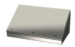
Saginaw operator consolet, NEMA 3R/4/4X/12/13, 20 x 30 x 13in (HxWxD), desktop or pedestal mount, 304 stainless steel, #4 brush finish, single-door, 1/4-turn semi-flush latch.
