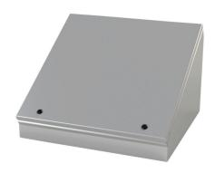
Saginaw operator consolet, NEMA 3R/4/12/13, 20 x 20 x 13in (HxWxD), desktop or pedestal mount, carbon steel, ANSI 61 gray, powder coat finish, single-door, 1/4-turn semi-flush latch.
