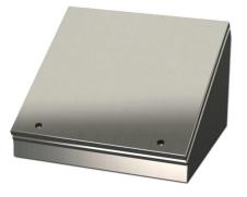
Saginaw operator consolet, NEMA 3R/4/4X/12/13, 20 x 20 x 13in (HxWxD), desktop or pedestal mount, 304 stainless steel, #4 brush finish, single-door, 1/4-turn semi-flush latch.
