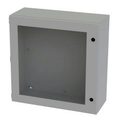
Saginaw Enviroline Junction series enclosure, NEMA 3R/4/12/13,  $20 \times 20 \times 8$  in (HxWxD), wall mount, carbon steel, ANSI 61 gray, powder coat finish, single-door, 1/4-turn semi-flush latch, polycarbonate window.
