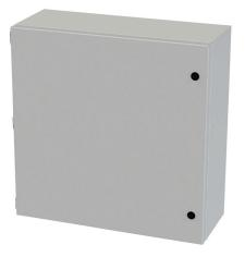
Saginaw Enviroline Junction series enclosure, NEMA 3R/4/12/13, 20 x 20 x 8in (HxWxD), wall mount, carbon steel, RAL 7035 light gray, powder coat finish, single-door, 1/4-turn semi-flush latch.
