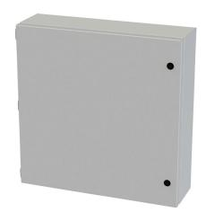
Saginaw Enviroline Junction series enclosure, NEMA 3R/4/12/13,  $20 \times 20 \times 6$  in (HxWxD), wall mount, carbon steel, RAL 7035 light gray, powder coat finish, single-door, 1/4-turn semi-flush latch.
