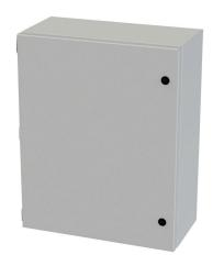
Saginaw Enviroline Junction series enclosure, NEMA 3R/4/12/13,  $20 \times 16 \times 8$  in (HxWxD), wall mount, carbon steel, RAL 7035 light gray, powder coat finish, single-door, 1/4-turn semi-flush latch.
