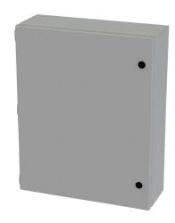
Saginaw Enviroline Junction series enclosure, NEMA 3R/4/12/13,  $20 \times 16 \times 6$  in (HxWxD), wall mount, carbon steel, ANSI 61 gray, powder coat finish, single-door, 1/4-turn semi-flush latch.
