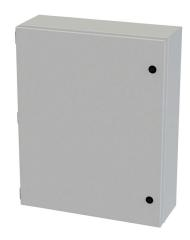
Saginaw Enviroline Junction series enclosure, NEMA 3R/4/12/13,  $20 \times 16 \times 6$  in (HxWxD), wall mount, carbon steel, RAL 7035 light gray, powder coat finish, single-door, 1/4-turn semi-flush latch.
