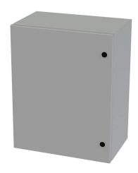
Saginaw Enviroline Junction series enclosure, NEMA 3R/4/12/13,  $20 \times 16 \times 10$  in (HxWxD), wall mount, carbon steel, ANSI 61 gray, powder coat finish, single-door, 1/4-turn semi-flush latch.
