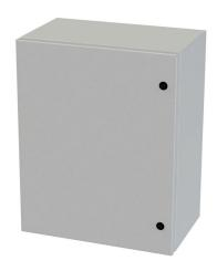
Saginaw Enviroline Junction series enclosure, NEMA 3R/4/12/13,  $20 \times 16 \times 10$  in (HxWxD), wall mount, carbon steel, RAL 7035 light gray, powder coat finish, single-door, 1/4-turn semi-flush latch.
