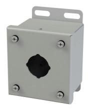
Saginaw pushbutton enclosure, 1 hole, 30mm, NEMA 4/12/13,  $4 \times 4 \times 3$  in (HxWxD), wall mount, carbon steel, ANSI 61 gray, powder coat finish, screw cover.
