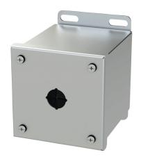
Saginaw pushbutton enclosure, 1 hole, 22mm, NEMA 4/4X/12/13, 4 x 4 x 5in (HxWxD), wall mount, 304 stainless steel, #4 brush finish, screw cover.
