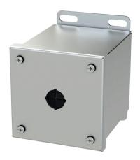
Saginaw pushbutton enclosure, 1 hole, 22mm, NEMA 4/4X/12/13,  $4 \times 4 \times 5$ in (HxWxD), wall mount, 316L stainless steel, #4 brush finish, screw cover.
