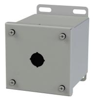
Saginaw pushbutton enclosure, 1 hole, 22mm, NEMA 4/12/13, 4 x 4 x 5in (HxWxD), wall mount, carbon steel, ANSI 61 gray, powder coat finish, screw cover.
