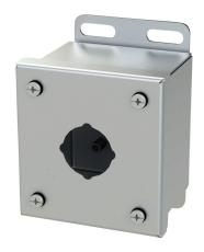
Saginaw pushbutton enclosure, 1 hole, 30mm, NEMA 4/4X/12/13, 4 x 4 x 3in (HxWxD), wall mount, 304 stainless steel, #4 brush finish, screw cover.
