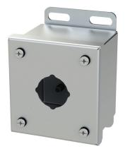
Saginaw pushbutton enclosure, 1 hole, 30mm, NEMA 4/4X/12/13, 4 x 4 x 3in (HxWxD), wall mount, 316L stainless steel, #4 brush finish, screw cover.
