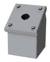
Saginaw pushbutton consolet, 1 hole, 22mm, NEMA 4/12/13, 4  $\times$  4  $\times$  5in (HxWxD), wall mount, carbon steel, ANSI 61 gray, powder coat finish, screw cover.
