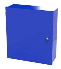
Saginaw enclosure, NEMA 1,  $18 \times 16 \times 6$  in (HxWxD), wall mount, with knockouts, carbon steel, precaution blue, powder coat finish, single-door, 1/4-turn semi-flush latch.
