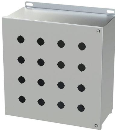
Saginaw pushbutton enclosure, 16 holes, 22mm, NEMA 4/4X/12/13, 12 x 12 x 6in (HxWxD), wall mount, 316L stainless steel, #4 brush finish, hinged screw cover.
