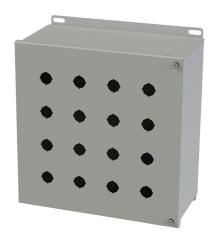
Saginaw pushbutton enclosure, 16 holes, 22mm, NEMA 4/12/13, 12 x 12 x 6in (HxWxD), wall mount, carbon steel, ANSI 61 gray, powder coat finish, hinged screw cover.
