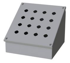
Saginaw pushbutton consolet, 16 holes, 22mm, NEMA 4/12/13,  $11 \times 11 \times 9$ in (HxWxD), wall mount, carbon steel, ANSI 61 gray, powder coat finish, screw cover, purchase subpanel separately.
