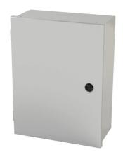
Saginaw enclosure, NEMA 1, 16 x 12 x 6in (HxWxD), wall mount, carbon steel, ANSI 61 gray, powder coat finish, single-door, 1/4-turn semi-flush latch.
