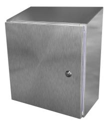
Saginaw sanitary enclosure, slope top, NEMA 3R/4/4X/12, 16 x 16 x 8in (HxWxD), wall mount, 304 stainless steel, #4 brush finish, single-door, 1/4-turn sanitary stainless steel latch.
