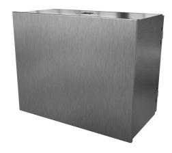
Saginaw HMI Enclosure, NEMA 3R/4/4X/12/13, 16 x 20 x 10in (HxWxD), suspension or pedestal mount, dual access, 304 stainless steel, #4 brush finish, screw cover front, single door rear, 1/4-turn semi-flush latch.
