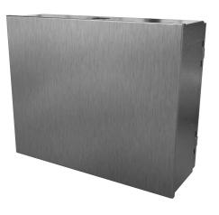
Saginaw HMI Enclosure, NEMA 3R/4/4X/12/13, 16 x 20 x 6in (HxWxD), suspension or pedestal mount, dual access, 304 stainless steel, #4 brush finish, screw cover front, single door rear, 1/4-turn semi-flush latch.
