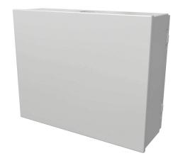
Saginaw HMI Enclosure, NEMA 3R/4/12/13, 16 x 20 x 6in (HxWxD), suspension or pedestal mount, dual access, carbon steel, RAL 7035 light gray, powder coat finish, screw cover front, single door rear, 1/4-turn semi-flush latch.
