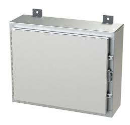
Saginaw enclosure, NEMA 3R/4/4X/12/13, 16 x 20 x 6in (HxWxD), wall mount, 304 stainless steel, #4 brush finish, single-door, stainless steel clamps, padlock hasp and staple.
