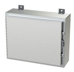
Saginaw enclosure, NEMA 3R/4/4X/12/13, 16 x 20 x 6in (HxWxD), wall mount, 316L stainless steel, #4 brush finish, single-door, stainless steel clamps, padlock hasp and staple.
