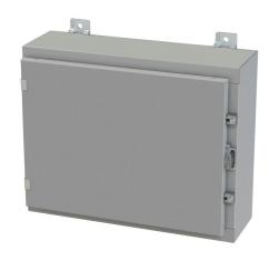
Saginaw enclosure, NEMA 3R/4/12/13, 16 x 20 x 6in (HxWxD), wall mount, carbon steel, ANSI 61 gray, powder coat finish, single-door, plated steel clamps, padlock hasp and staple.
