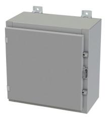
Saginaw enclosure, NEMA 3R/4/12/13, 16 x 16 x 8in (HxWxD), wall mount, carbon steel, ANSI 61 gray, powder coat finish, single-door, plated steel clamps, padlock hasp and staple.
