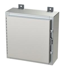
Saginaw enclosure, NEMA 3R/4/4X/12/13, 16 x 16 x 6in (HxWxD), wall mount, 304 stainless steel, #4 brush finish, single-door, stainless steel clamps, padlock hasp and staple.
