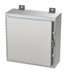
Saginaw enclosure, NEMA 3R/4/4X/12/13, 16 x 16 x 6in (HxWxD), wall mount, 316L stainless steel, #4 brush finish, single-door, stainless steel clamps, padlock hasp and staple.
