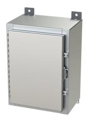
Saginaw enclosure, NEMA 3R/4/4X/12/13, 16 x 12 x 8in (HxWxD), wall mount, 316L stainless steel, #4 brush finish, single-door, stainless steel clamps, padlock hasp and staple.
