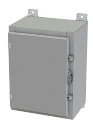
Saginaw enclosure, NEMA 3R/4/12/13, 16 x 12 x 8in (HxWxD), wall mount, carbon steel, ANSI 61 gray, powder coat finish, single-door, plated steel clamps, padlock hasp and staple.
